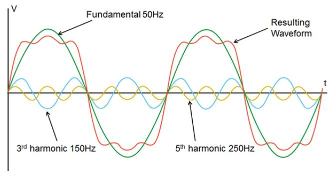
Capacitor banks themselves do not cause harmonics, but they can cause resonance, which amplifies existing harmonics in the system. Careful selection of PFC is therefore required, with knowledge of the type of loads so that this is avoided. Blocking reactors (inductance in series with the capacitor banks) tuned below either the 3<sup>rd</sup> or 5<sup>th</sup> harmonic are available, depending on the system load profile.
