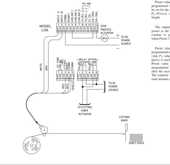
Preset value  $P_1$  (*Process count*) is programmed for the first length to be cut for the order and Preset value  $P_2$  (*Process count*) for the second length.
